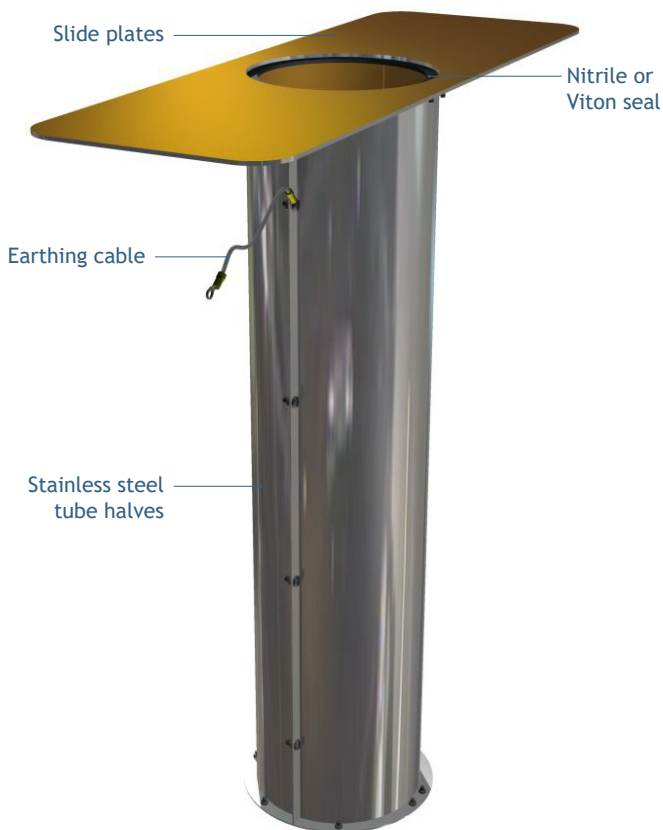
Single guide pole sleeve
